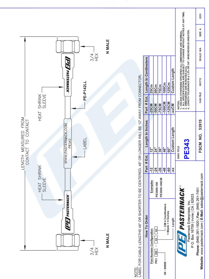
PE343-150CM CAD Drawing N Male to N Male Low Loss Test Cable 150 CM Length Using PE-P142LL Coax, RoHS
